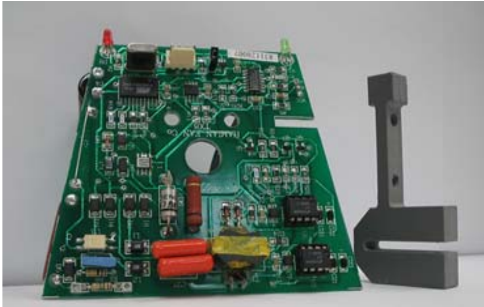
Figure 1: Transmitter board and the IR mounting assembly
