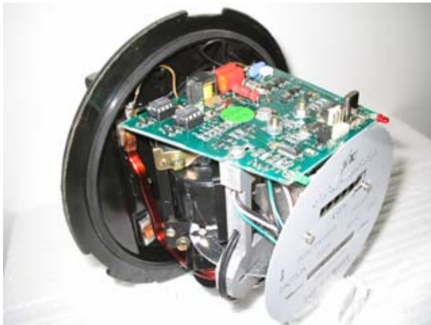
Figure 1: Transmitter board and the IR mounting assembly
